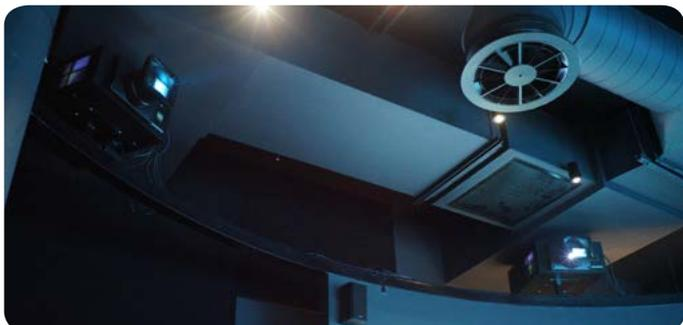
A Digital Projection HIGHlite Laser 11k (WUXGA 1920 1200) was chosen to provide an active stereo 3D, 18.8m wide (240 degree) Cylindrical Panoramic projection 4-channel warp and blend solution.
